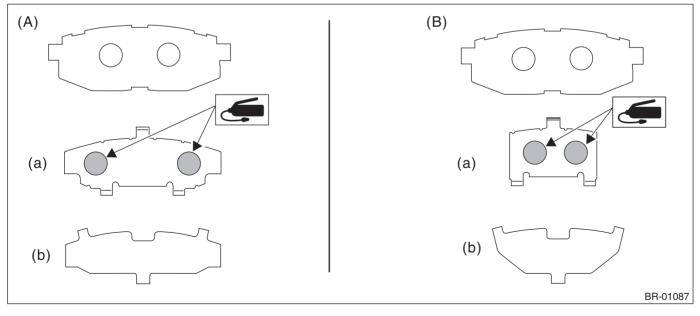
(A) Pad - disc brake rear outer (B) Pad - disc brake rear inner
